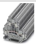
Double-level terminal block, connection method: Screw connection, cross section: 0.14 mm² - 4 mm², AWG: 26 - 12, width: 5.2 mm, color: gray, mounting type: NS 35/7,5, NS 35/15
